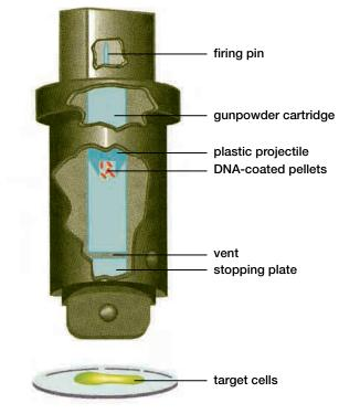
**Figure 9.24** Sanford's DNA particle gun fires microscopic metal pellets coated with foreign DNA. The pellets are attached to a plastic projectile that is shot through the gun chamber. When the projectile hits the stopping plate, the pellets are torn off and carried into the plant cells and some of their nuclei. The foreign DNA may then be incorporated into the plant DNA.
