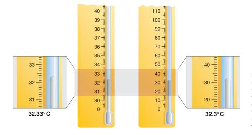
Figure A3.1 A temperature measurement made using the thermometer on the left will have more significant digits, hence more certainty, than a measurement made using the thermometer on the right. One way to avoid ambiguity is to express numbers using scientific notation. Thus, in  $5 \times 10^6$  bacteria, it is clear that there is one significant digit.
